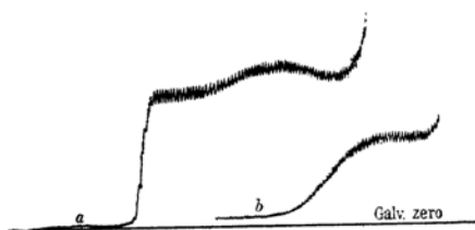
Fig. 5.—Polarograms of Pb^{2+} ion and H^+ ion: a, Pb^{2+} ion in KOH solution; b, 0.52 millimole HCl—0.1 \times KCl.
